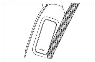
If your vehicle has a side impact airbag for the driver it will say AIR BAG on the airbag covering on the side of the driver's seatback closest to the door.
